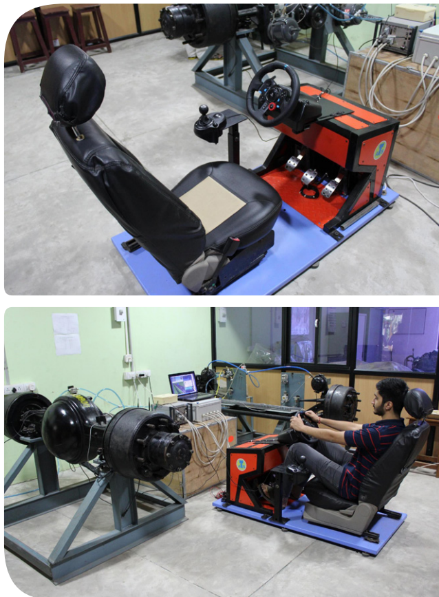
Fig. 2: Hardware-in-loop testing facility of a heavy vehicle
